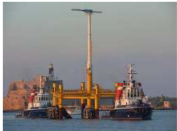
**Figure 7: Blue H floating wind platform**
